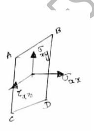
In above figure plane ABCD is 'X-plane'. There is a normal force and two shear stress in a plane of '3-D structure'. The normal stress in plane ABCD is noted as  $\sigma_{xx}$ . Similarly, shear stress  $\tau_{xy}$  in y-direction and  $\tau_{xz}$  in z-direction.
