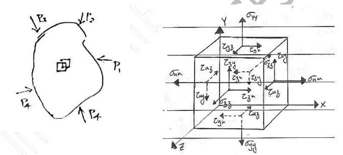
There are 3-planes in a cubical partial (X, Y, Z). In each plane (one normal stress and two shear stress).
