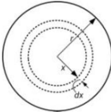
The conductor has a radius of  $r$  and carries a current  $I$ . Ampere's law states that the magneto motive force (mmf) in ampere-turns around a closed path is equal to the net current in amperes enclosed by the path. We then get the following expression
