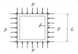
The deformed shape is a square of dimension  $L - 2 \delta$ . If L = 2 m and  $\delta = 0.001 \text{ m}$ , the Poisson's ratio of the plate material is
