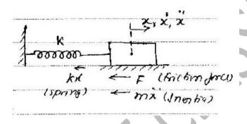
Here Mass is moving from LHS to RHS and initial displacement is  $-X_0$
