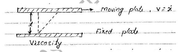
Consider two plates are separated by fluid film of thickness t. The upper plate is allowed to move parallel to the fixed plate with a velocity  $\dot{x}$ . The net force F required for maintaining the velocity  $\dot{x}$  of the plate is expressed as;
