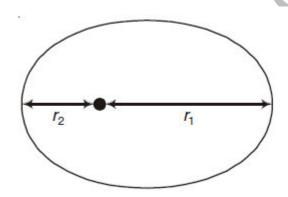
$$e = \frac{r_1 - r_2}{r_1 + r_2}$$
