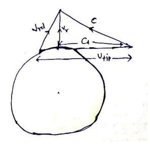
$$V_{rel} = \sqrt{V_r^2 + (U_{tip} - C_t)^2}$$
