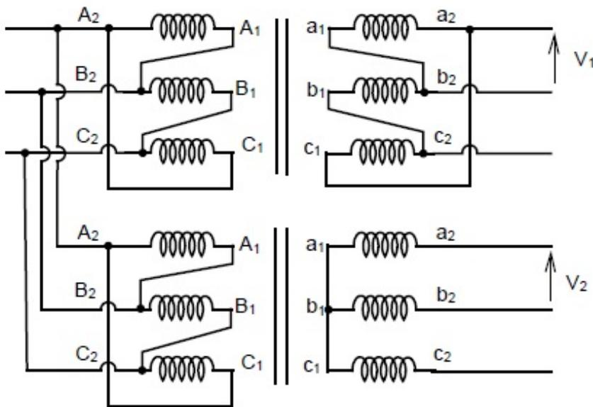
The phase difference (in degree) between voltages  $V_1$  and  $V_2$  is \_\_\_\_\_.
