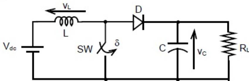
Under steady state operating conditions, the average voltage across the inductor and the capacitor respectively, are
