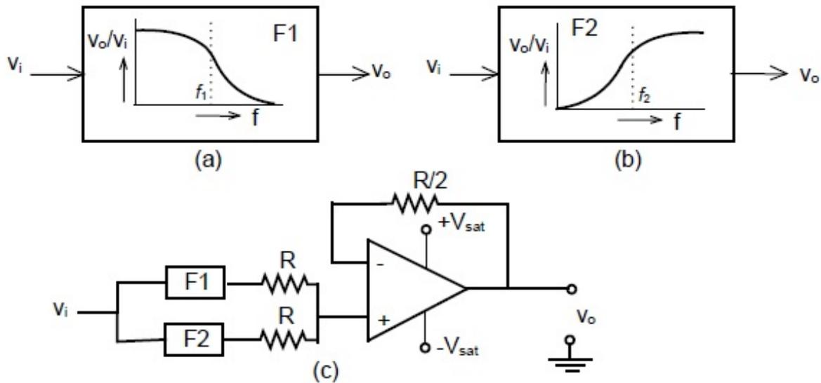
The cut-off frequencies of F1 and F2 are  $f_1$  and  $f_2$  respectively. If  $f_1 < f_2$ , the resultant circuit exhibits the characteristic of a
