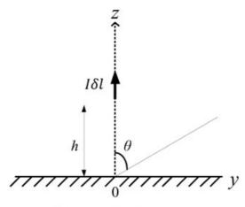
Infinite conducting plane
