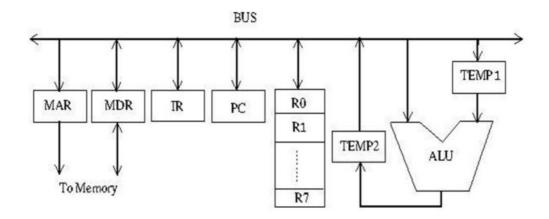
Consider an instruction:  $R0 \leftarrow R1 + R2$ . The following steps are used to execute it over the given data path. Assume that PC is incremented appropriately. The subscripts r and w indicate read and write operations, respectively.
