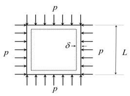
The deformed shape is a square of dimension  $L-2\delta$ . If L=2 m and  $\delta=0.001$  m, the Poisson's ratio of the plate material is \_\_\_\_\_
