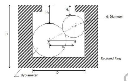
The distance  $H_2$ =35.55 mm and  $H_1$ =20.55 mm. The diameter (D, in mm) of the ring gauge is \_\_\_\_\_
