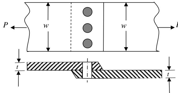
width of the plate  $w = 200 \text{ mm}$ , thickness of the plate  $t = 5 \text{ mm}$ , number of rivets  $n = 3$ , diameter of the rivet  $d_r = 10 \text{ mm}$ , diameter of the rivet hole  $d_h = 11 \text{ mm}$ , allowable tensile stress of the plate  $\sigma_p = 200 \text{ MPa}$ , allowable shear stress of the rivet  $\sigma_s = 100 \text{ MPa}$  and allowable bearing stress of the rivet  $\sigma_c = 150 \text{ MPa}$ .
