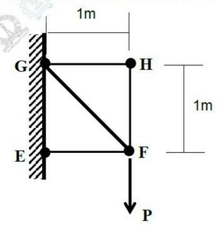
A rigid frame grips on to a steel wall as shown using a powerful magnet at the top support G and with a roller support at E. EF is horizontal. A man stands on the platform attached to the frame 1m away from the wall as shown. Assume the frame and magnet assembly to be of negligible weight and the mass of the man to be 80kg. The magnitude of the reaction (in Newtons) exerted by the frame onto the steel wall due to the weight of the man is \_\_\_\_\_\_.
